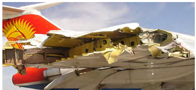
Fig. 11. Details of the damaged right wing of the Tu-154M EX-85718, which struck the parking KC-135R tanker.
