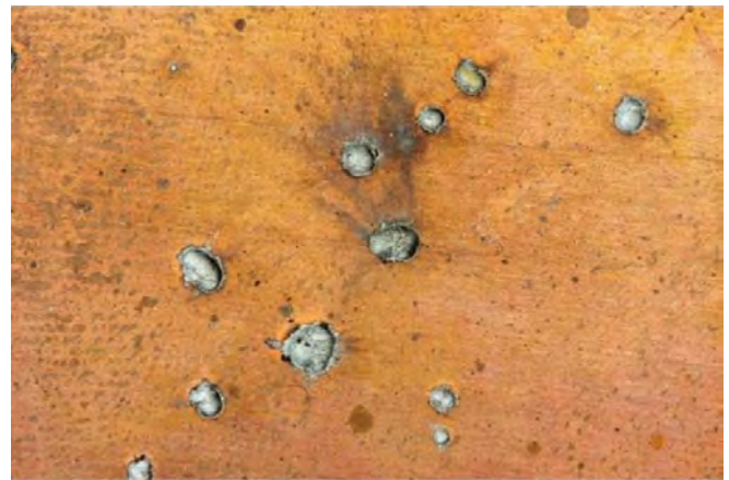
Fig. 35. Experimental explosive cladding: aluminum deposited on a copper sheet. Craters are formed explosively [14].
