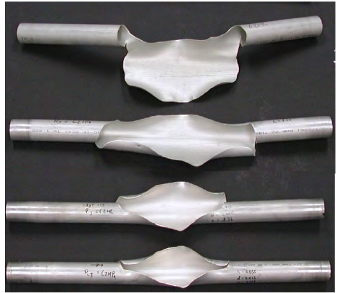
Fig. 29. Examples of confined ruptures of experimental aluminum tubes under internal gaseous detonation [28].
