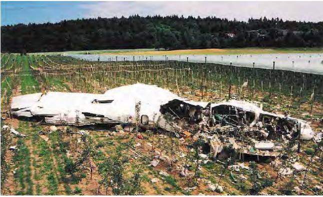
Fig. 5. The forward fuselage section of the Tu154M RA-85816 (Überlingen mid air collision July 1, 2002) found at apple plantation near Brachenreuthe (Lake Constance) [6].
