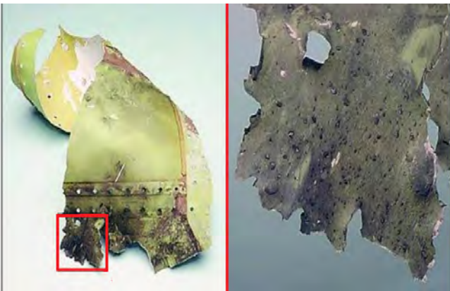
Fig. 32. Good example of explosive signature that shows pulled rivets, staining, microcraters, petaled hole, rolled edges (curl) and gas wash in the skin of an aircraft fuselage [17].
