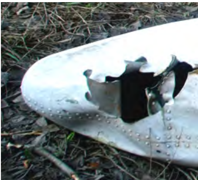
Fig. 33. Petaled hole with rolled edges in a wing part (probably wing fairing) of the Tu-154M PLF 101 found near crash site. This hole is not a full evidence of explosion because no other symptoms of explosion as, for example, tensile rivet failure, staining, impact craters, etc., are visible. Source: http://inapcache.boston.com/universal/site_graphics/blogs/bigpicture/poland_04_12/p03_22969387.jpg
