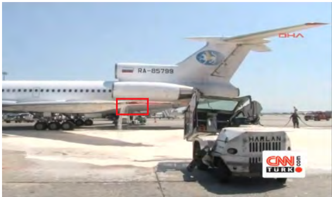
Fig. 44. Tu-154M RA-85799 and luggage truck after collision at Istanbul Ataturk airport on July 27, 2011. Source: http://www.euromag.ru/turkey/11679.html .
