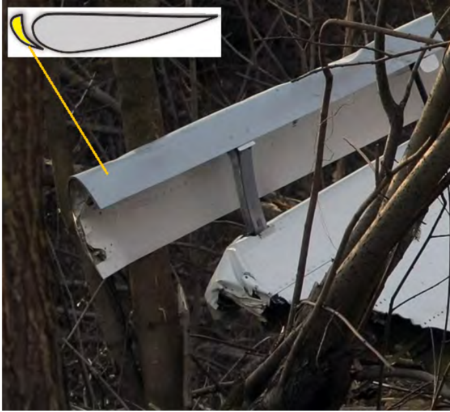
Figure 3.15: Tip of the left wing of the Tu154M No 101 after air crash. The main body of the wing has been cut off while the slat is intact.
