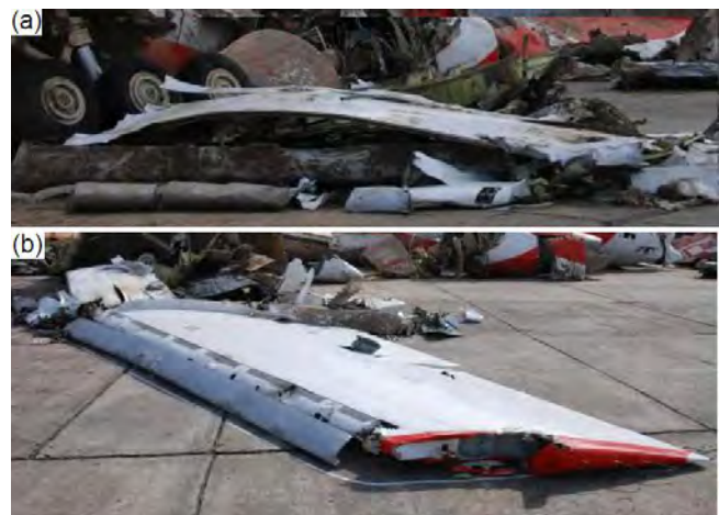
Figure 2.5: Left wing on the wreckage storage site: (a) effect of shock wave penetrating inside the wing [45]; (b) severed tip of the wing [16].
