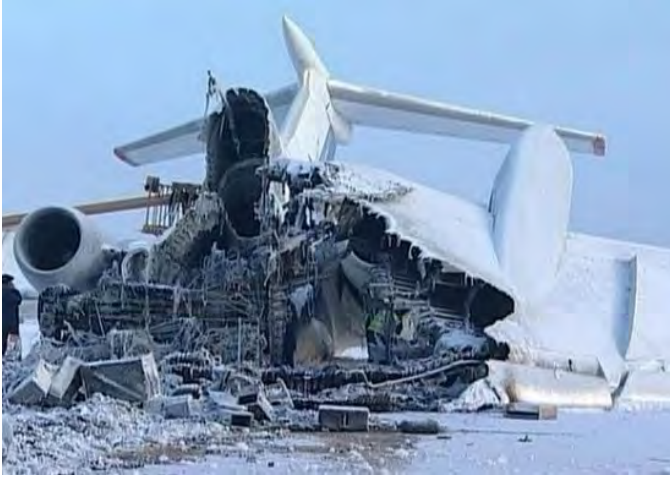
Figure 1.12: Tail part of Tu-154B2 RA-85588 after fire at Surgut airport on January 1, 2011 [30].
