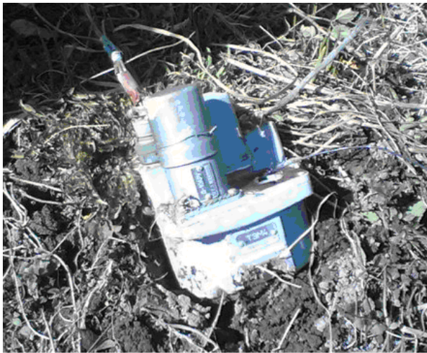
Figure 1.19: Electromagnetic brake TEM-4 for flap control found several meters behind the famous birch tree. Source: http://www.waronline.org
